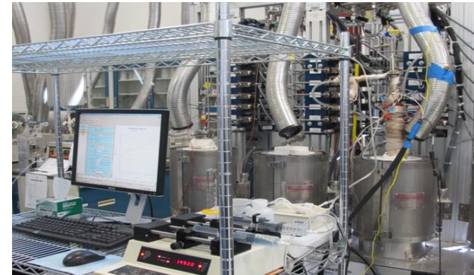
Integrated SOFC test system
